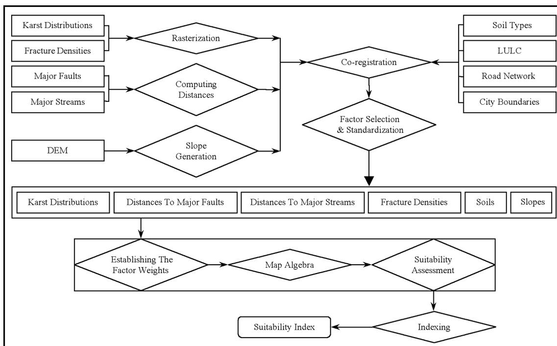
Figure 2. Modeling methodology developed for the assessment of site suitability.
